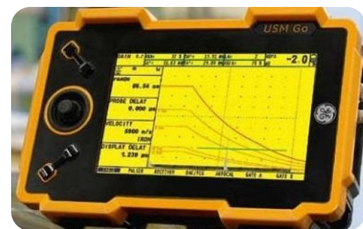
USM36 GE Inspection / Krautkramer/Ultrasonic flaw detector
