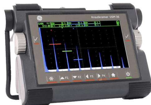
USM36 GE Inspection / Krautkramer/Ultrasonic flaw detector
